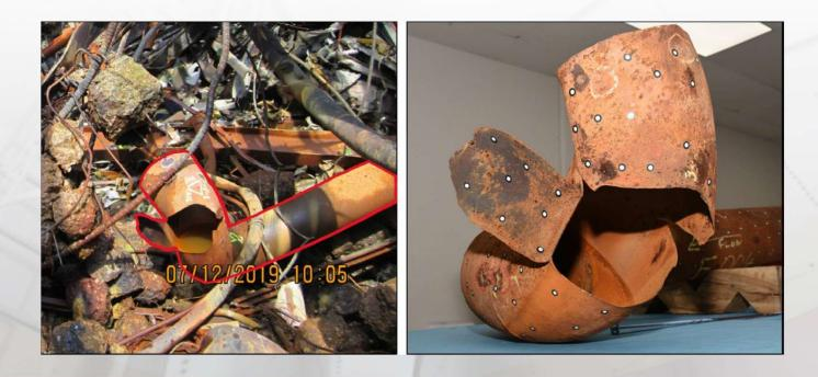
Contributing to the incident was the lack of requirements by the American Petroleum Institute, Sunoco, and PES, to inspect all existing carbon steel piping circuit components to ensure they could safely operate in HF service.
