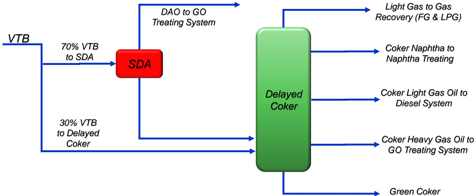
From the Resid Pool, the residue is sent to either the SDA or directly to the Delayed Coker. In this study, 70% is sent to the SDA and 30% to the DCU directly. The pitch or asphalt produced in the SDA is fed to the Coker. All the Coker products and the SDA DAO are then sent to downstream processing systems.
