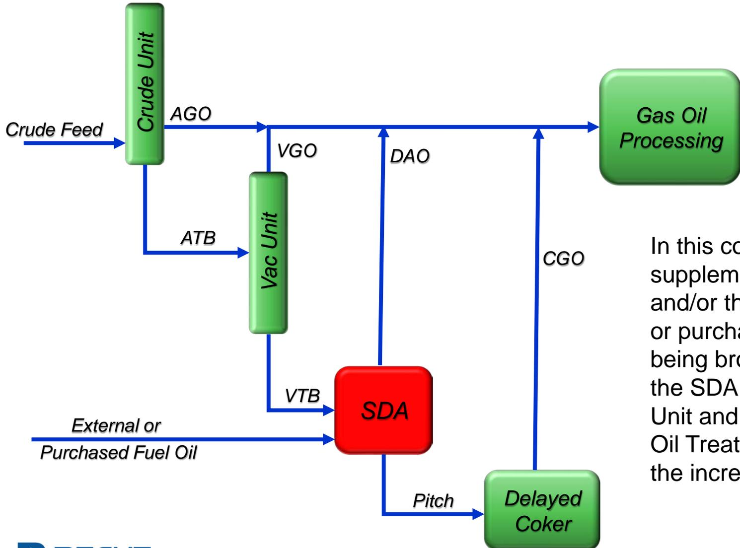
In this configuration, the SDA is being used to supplement or unload capacity in the Vacuum Unit and/or the Delayed Coker. Additionally, an External or purchased fuel oil (containing cutter and resid) is being brought into the refinery and preprocessed in the SDA, which further unloads both the Vacuum Unit and Delayed Coker. Here again, the Heavy Gas Oil Treating system must be reviewed/evaluated for the increase in capacity.
