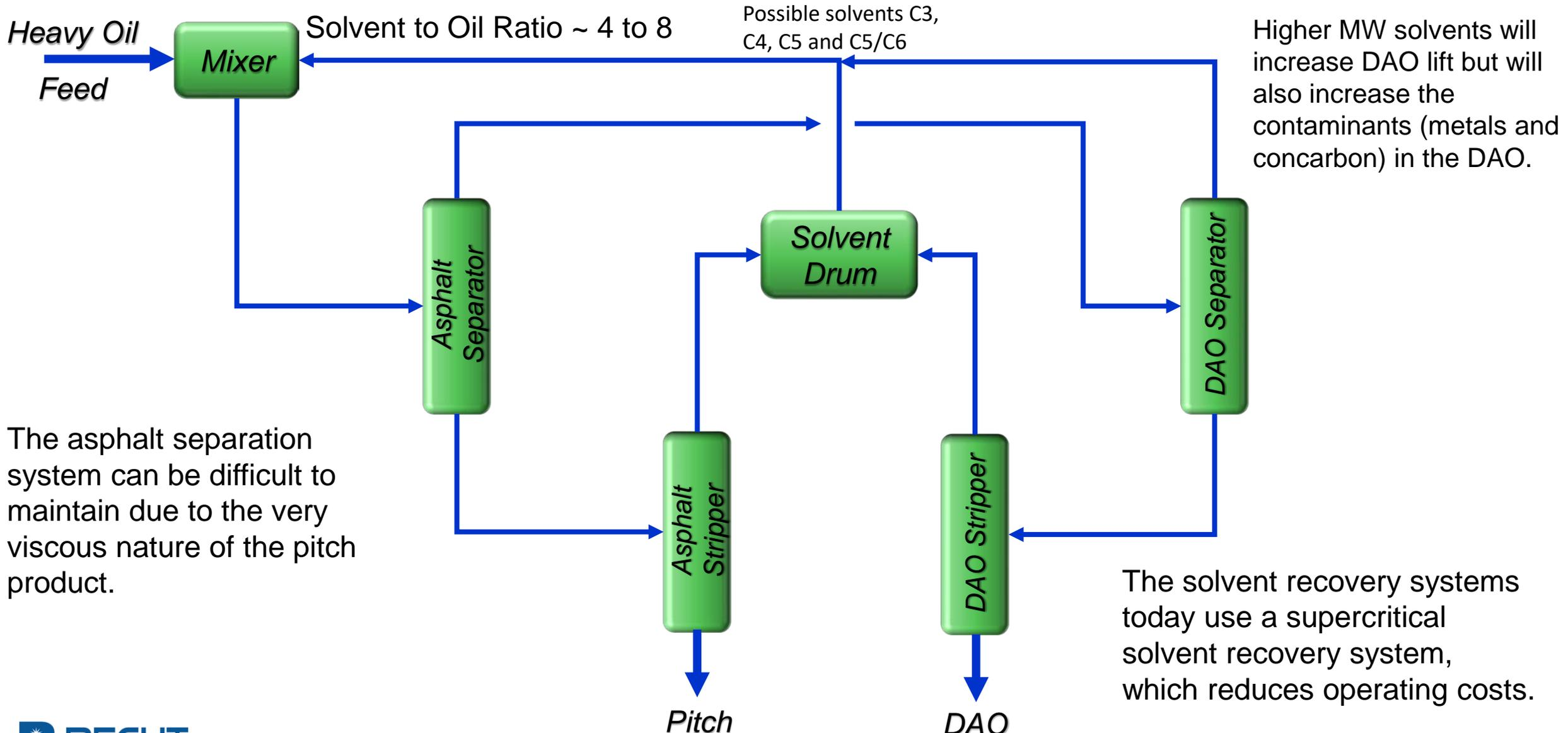
The asphalt separation system can be difficult to maintain due to the very viscous nature of the pitch product.
