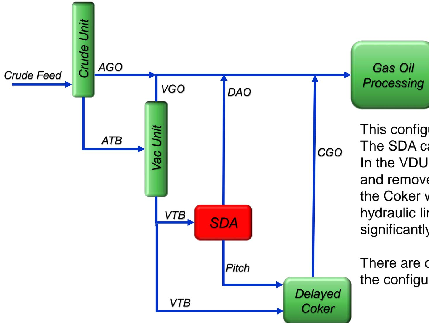
This configuration is what is most frequently seen. The SDA can support both the VDU and/or the DCU. In the VDU it can address poor cut point operations and remove some load from the Coker. Unloading the Coker will improve the fired heater capacity and hydraulic limitation. However, the SDA does not significantly reduce the amount of coke produced.
