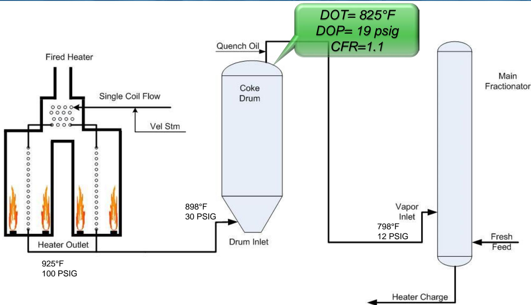
The Delayed Coker's operations were kept constant and reflect a typical Delayed Coker. The Coker is a small (~25,000 BPD), 2 drum (26ft ID) Coker, operating with approximately a 16-hour fill cycle.
