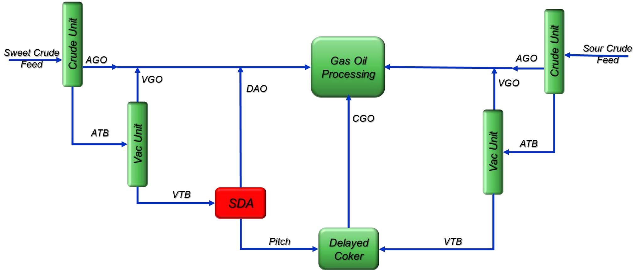
This configuration addresses crude incompatibility problems in the coker. More paraffinic material is removed from the Coker feed, allowing the Coker to process feeds that will not have solubility problems. Additionally, this configuration will unload the Delayed Coker fired heat further improving the Delayed Coker run length and reliability.
