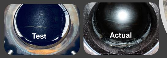
A hot rubberized tar material with similar properties to coke was poured into the MOGAS valve
