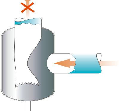
Internal Duct Buckling obstructing Gas Flow
