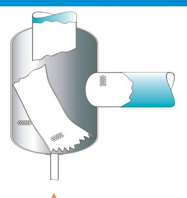
Internal Duct Rupture (Thermal Shock)
