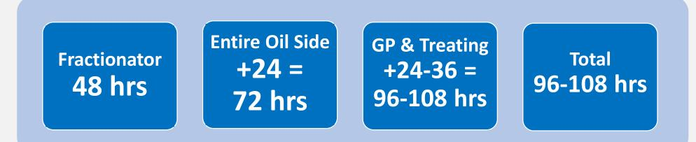
But, a novel approach in February 2019 resulted in an *entire* FCCU ready for maintenance in **~58 hours** from oil out.
