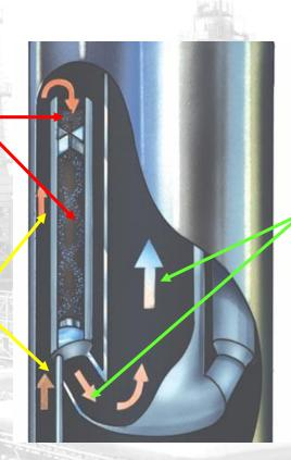
3. Gas flow out bottom of droplet separator tubes and into bottom of stack and up stack
