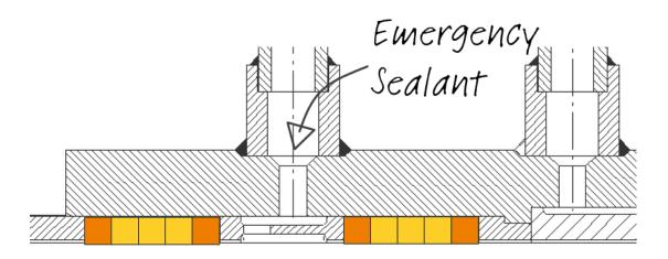
A graphite based special compound can be injected in the Emergency Sealant Port using an high pressure hand pump, in order to stop or decrease the leakage in case of safety concern.
