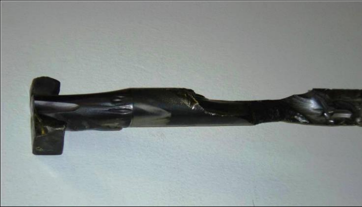
Stem damage due to excessive packing gland purging
