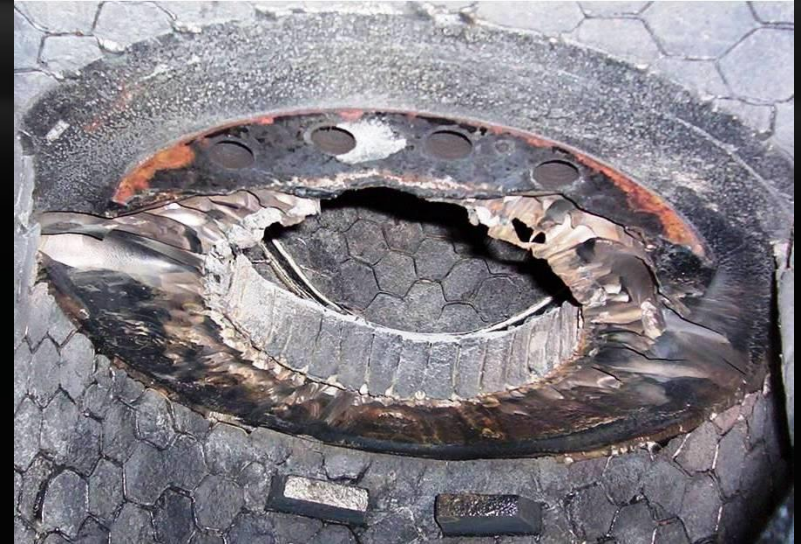
Seating Plate damage due to excessive purging
