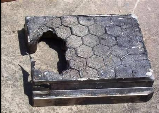
Disc damage due to excessive packing gland purging
