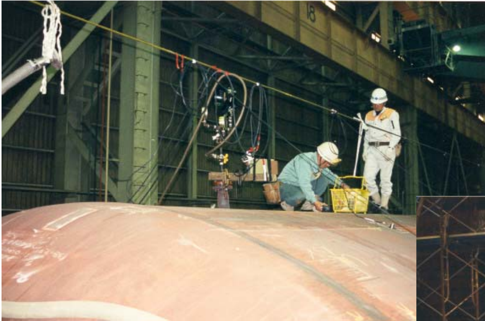
Sumitomo UT inspectors checking AET indication
