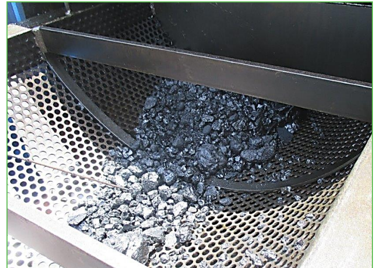
Results: loose coke for ease of removal. (Pictured: coker strainer basket)
