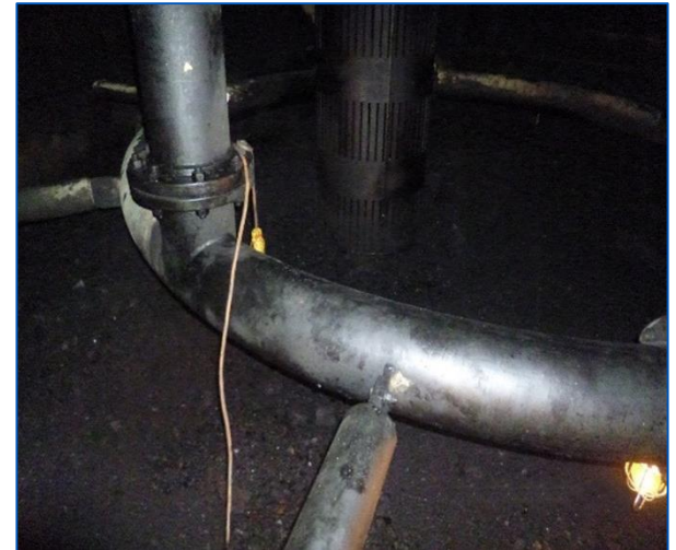
Bottom distributor was accessible and completely unplugged
