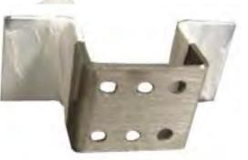
Each probe with its corrosion products was weighted. Corrosion layer was removed as per ASTM G1 and each probe was weighted again without the corrosion layer.
