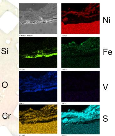
Example: Electron image and X ray dot maps of the corrosion product formed on 5923 alloy located in test plate 1
