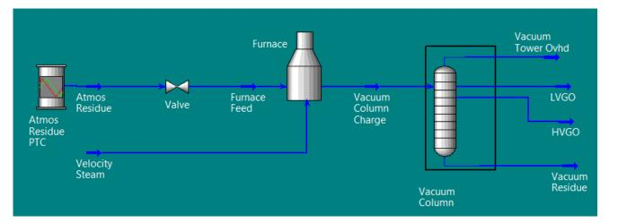
KBC has developed a detailed heater fouling model
