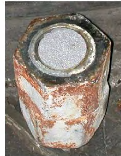
Broken Anchor Bolt W/2 Nuts
