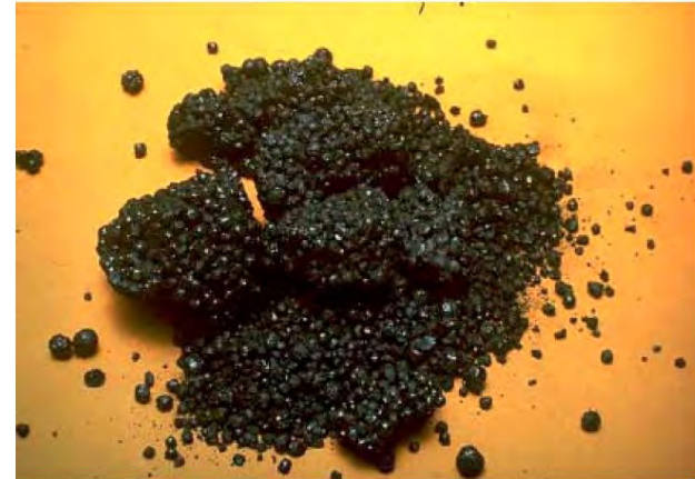
Shot Coke (Partially crushed to show shot structure)
