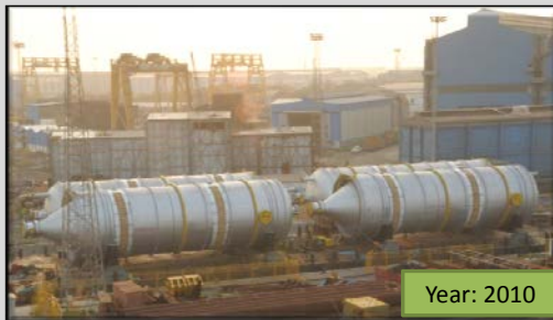
Coke Drum: CB&I Process – 8.0 m ID, 240 MT Each, 04 Nos
