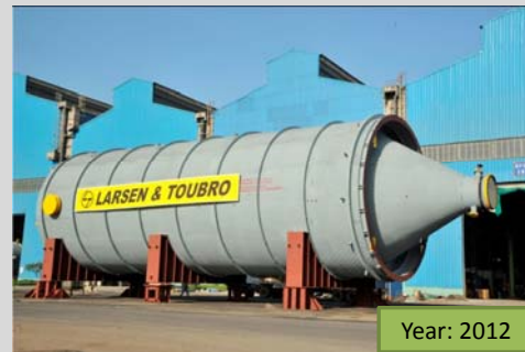
Coke Drum: Petrobras Process – 8.9 m ID, 245 MT Each, 16 Nos,
