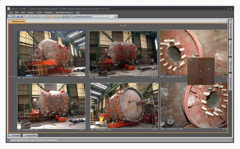
The features to be inspected are automatically detected on the photographs.
