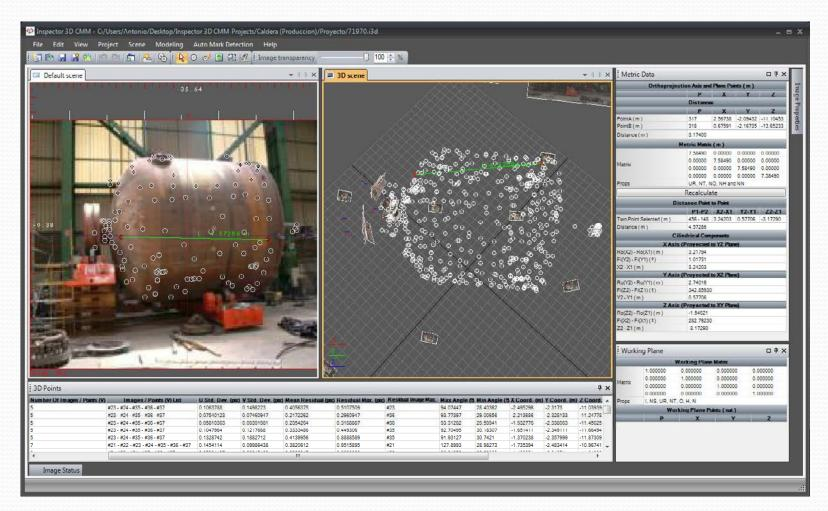
Any 2D/3D measurement can be carried out using both the 3D model and the set of images.
