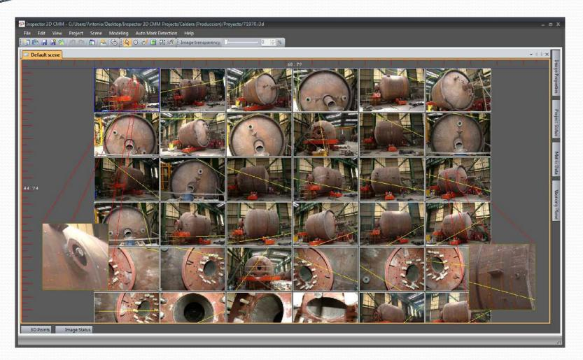
A set of images is taken during the manufacturing process. No need to stop such process
