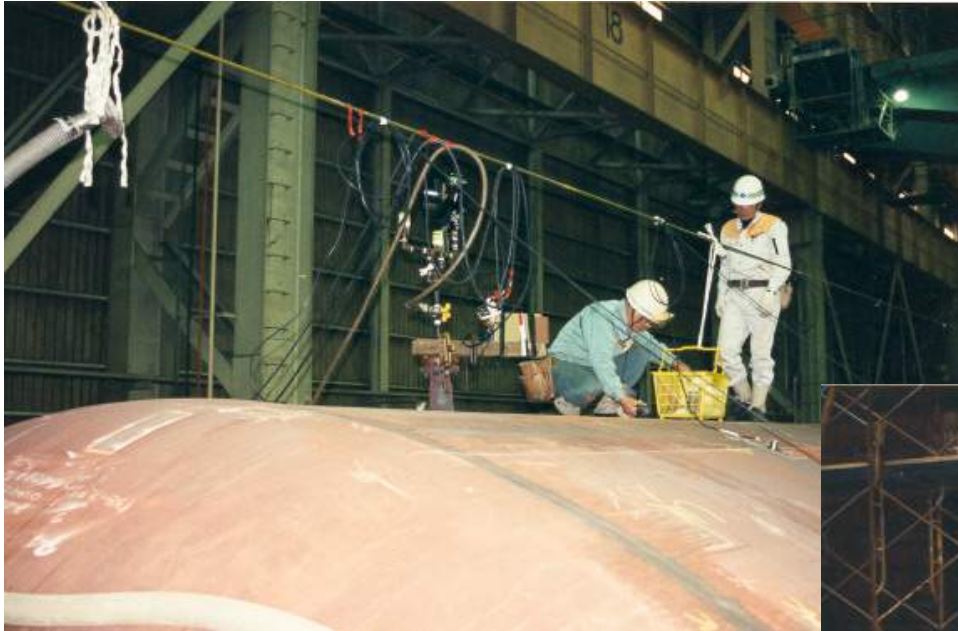
Sumitomo UT inspectors checking AET indication
