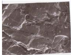
Delayed Coker Furnace Tube Deposits
