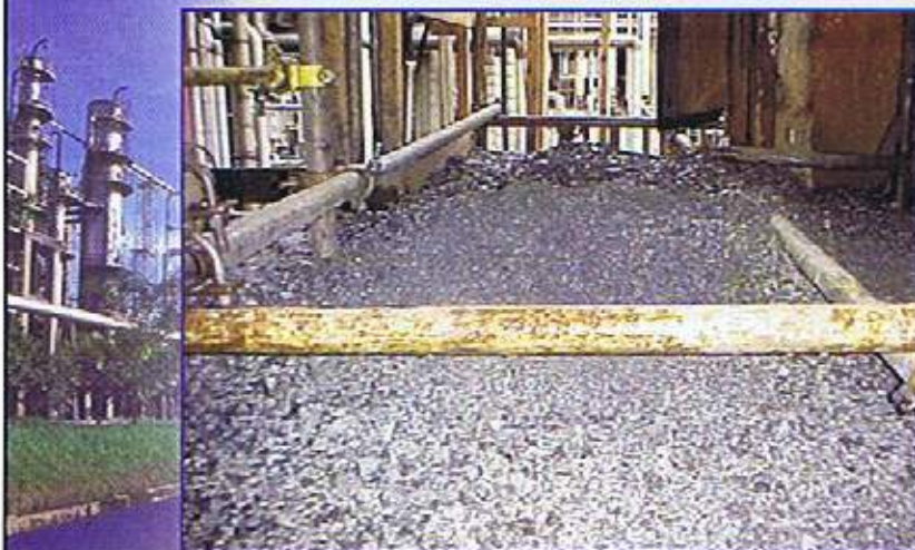
Deposits removed after heater decoking
