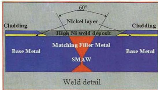
Fig. 3 — A typical weld detail.
