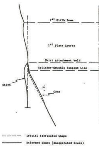
Fig. 7 Deformation pattern of vessels in heavily cyclic service
