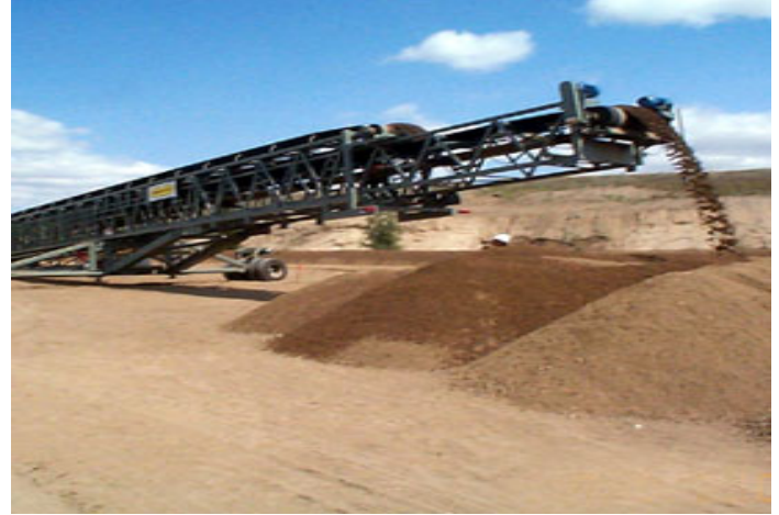
Example of the stacking pattern for an extendable circular stacker
