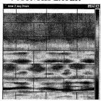
Carbon Steel - Note bulge growth between weld seams
