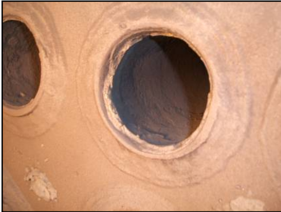
Figure 11. WHB Tubesheet Joint After 25 Years Service (From an Ortloff licensed unit, case history SRU-1)
