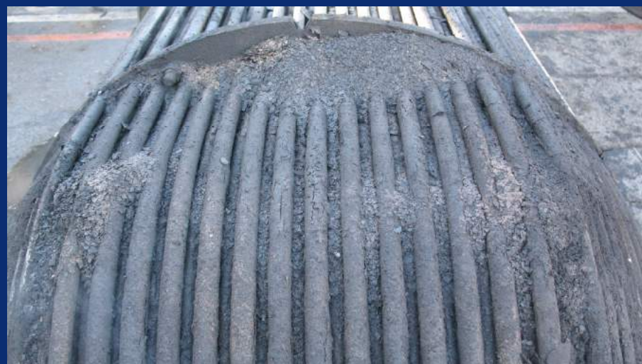
Packed with of Iron sulfide scale at top of bundle (E-535B)
