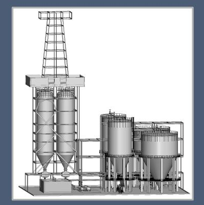
TRIPLAN Technology GmbH Essostrasse 16 76189 Karlsruhe Germany **Closed Coke Slurry System**
