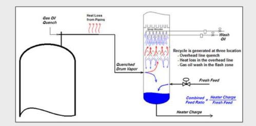
• Having large number of Trays in flash zone wash section requires additional wash too keep trays wet and avoid coking. This contributes to Recycle
