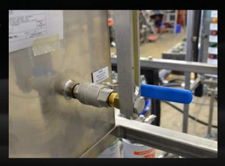
Reservoir fabricated from 3mm sheet 304SS
