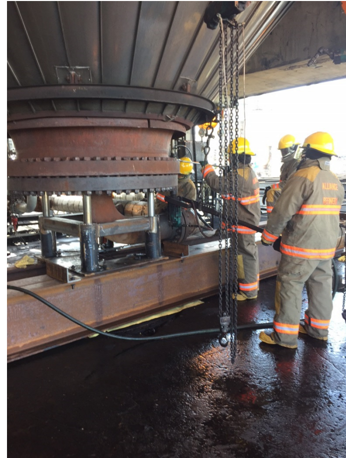
Test on water-filled sister drum. Device held full load with excellent control of hydraulics.
