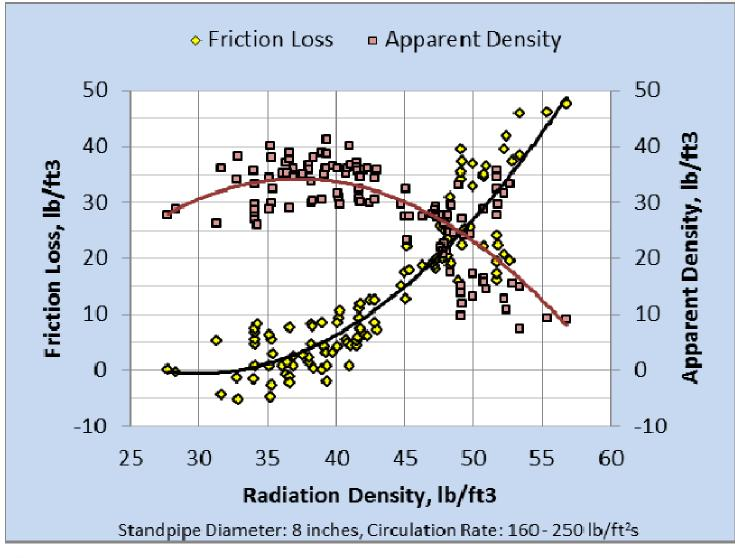
Minimum Fluidization Density: 45 lb/ft3, Loose Packed Density: 45 lb/ft3, Packed Density: 50 lb/ft3
