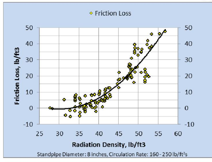
Minimum Fluidization Density: 41.0 lb/ft3, Loose Settled Density: 45.2 lb/ft3, Packed Density: 50 lb/ft3 John Matsen, "Some Characteristics of Large Solids Circulation Systems", Fluidization Technology, 1976
