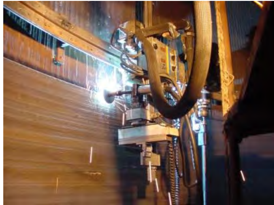
Automated Welding System Applying Inconel 625 in Pressure Vessel
