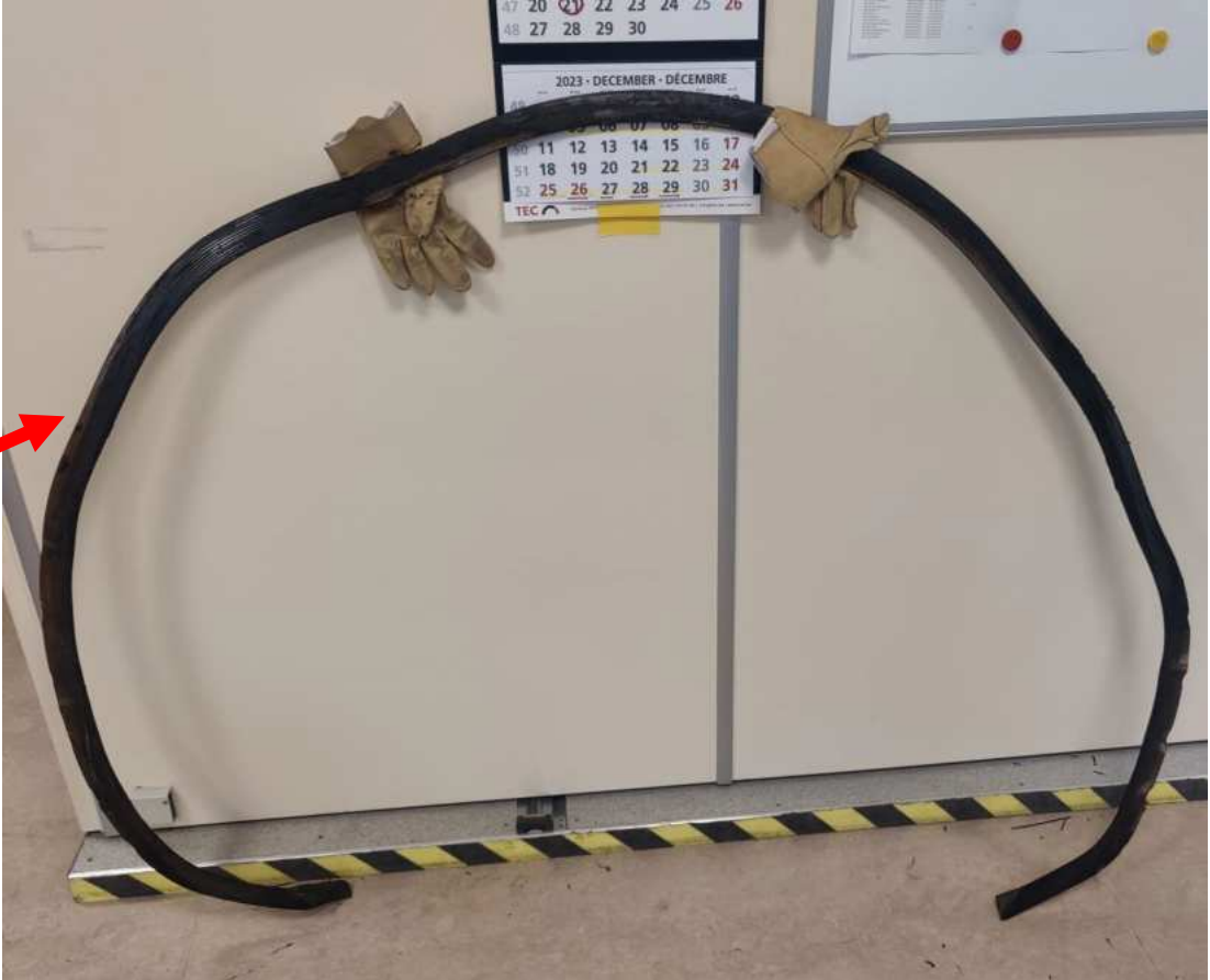
Missing gasket section introduces potential for larger leak vs historical flange leakage experience
