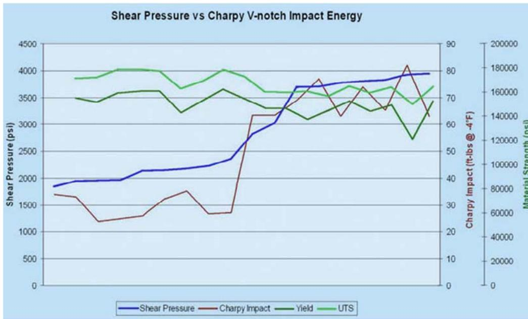
**Shear strength; Impact Strength governs over Material Strength.**
