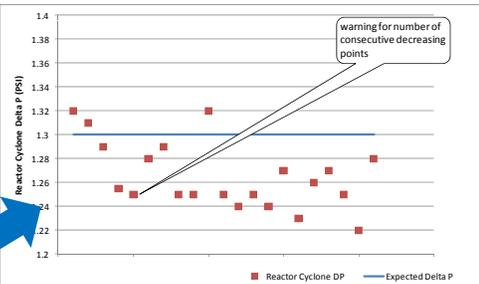
Reactor cyclone operation shown here for 3 weeks of operation
