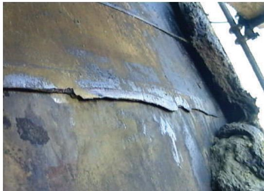
Thermally induced fatigue crack in circ. weld of a coke drum
