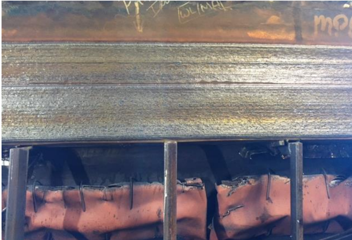
Machine Applied Knuckle Weld Deposit Completely Covering Casting Insert
