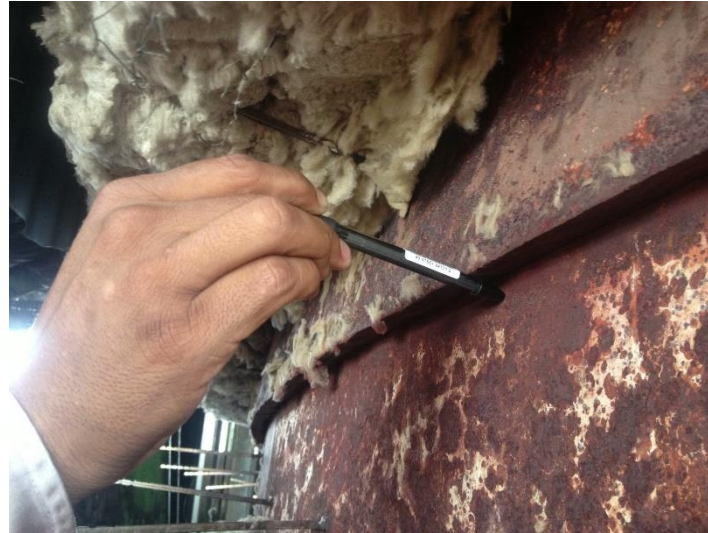
Skirt Attachment Cracking
