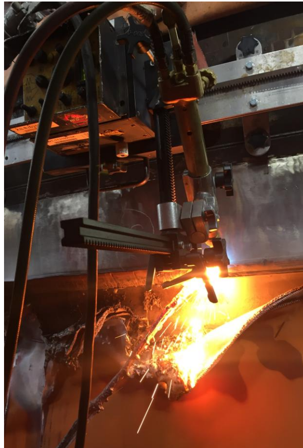
Machine Torch Cutting of the Weld Bevel
