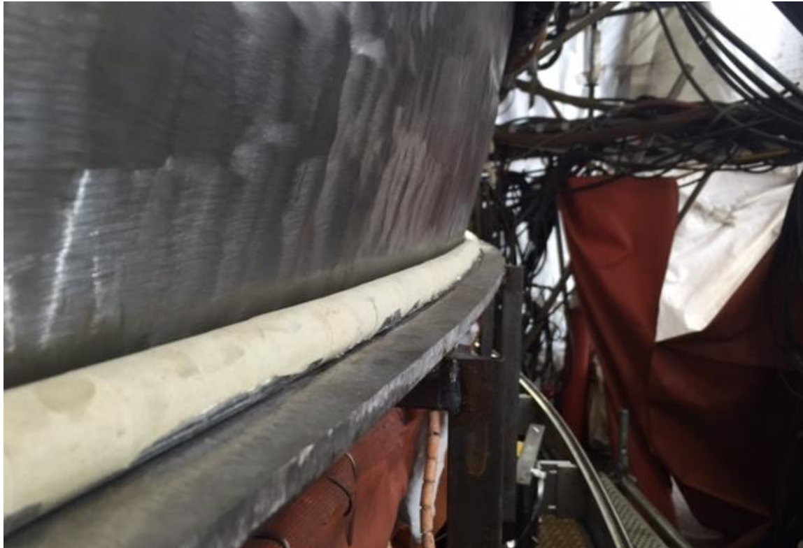
Casting Insert (White) and Welding Shelf
