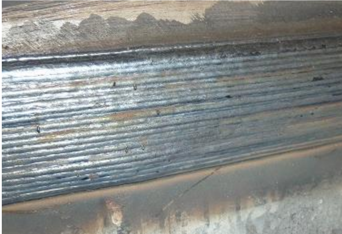
Appearance of ER70S-B2L Deposit (Two Layers)
