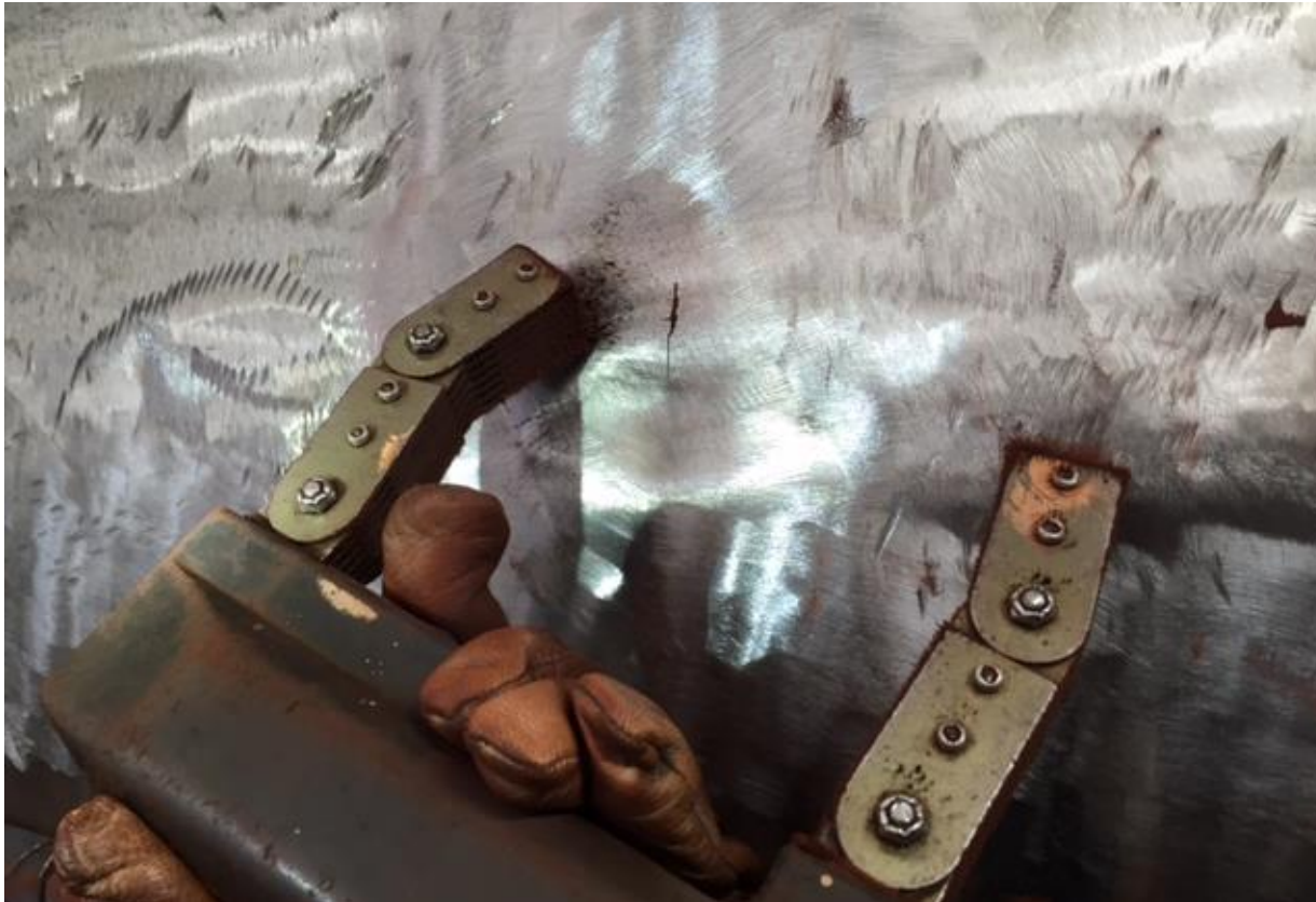
Magnetic Particle Inspection of Coker Vessel Base Material (Showing Vertically Aligned Crack)
