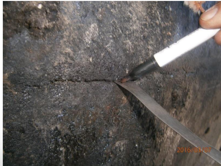
Pressure Boundary Cracking
