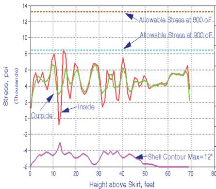
Axial Stress For Bulged Drum at 324 deg Profile (95)
