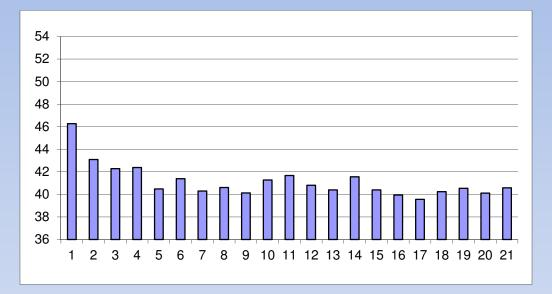
Monitoring after a few weeks indicated deterioration had pretty much leveled off. This was attributed to reduced thermal cycling and starting stresses due to running motor constantly.
