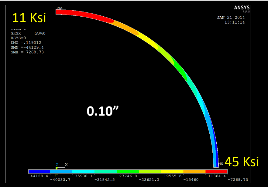
Effect of Gasket Seating Surface Out of Flatness on Gasket Stress
