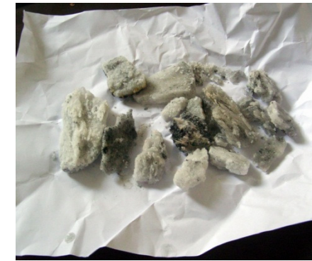
Solid material carried out by clean flue gas
