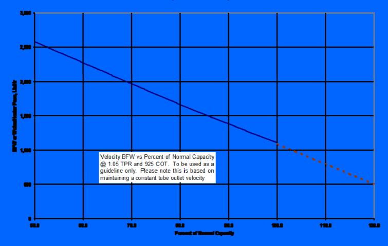
Each heater should have a velocity injection medium curve developed for the feedstock to be processed in the tube size installed
