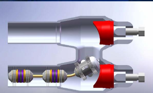
Plug headers as pictured will allow for Quest Integrity Group's FTIS intelligent pig inspection process
