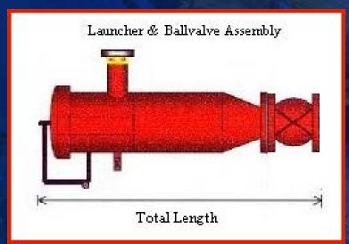
Length 4" Assembly - 56" 6" Assembly - 66 3/4" 8" Assembly - 68 3/4"
