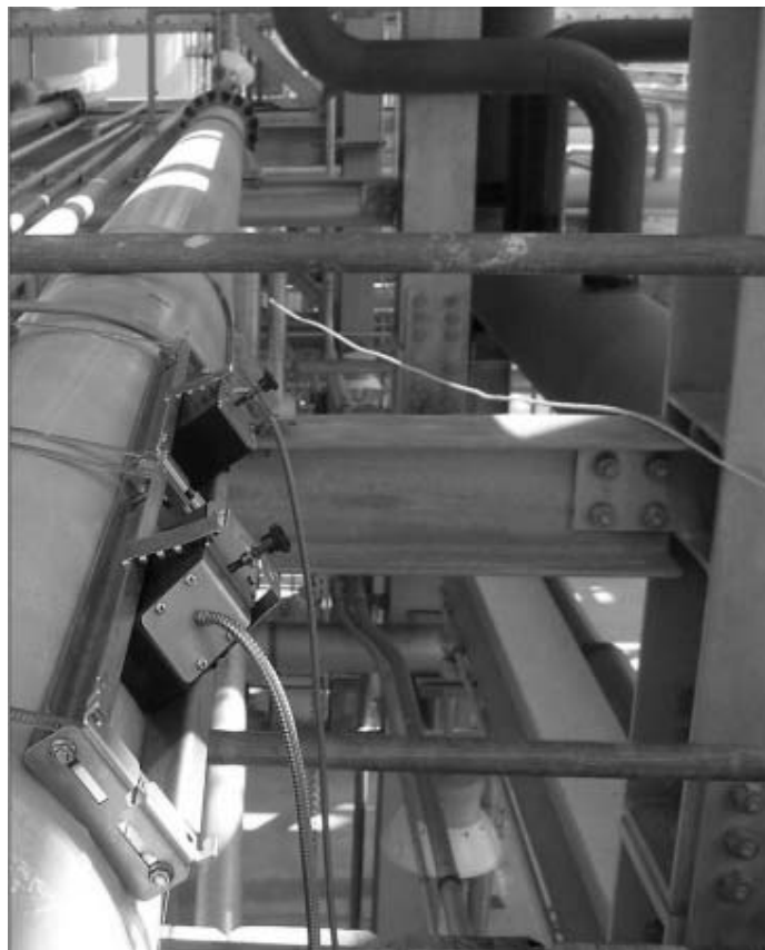
Fig. 12 : Ultrasonic Clamp-On Measurement
