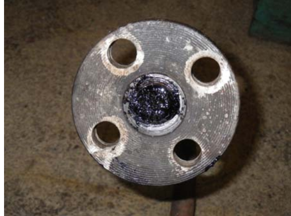
Fig. 5 : DP Assembly Removed (Left) and Impulse Lines Blocked (Right)
