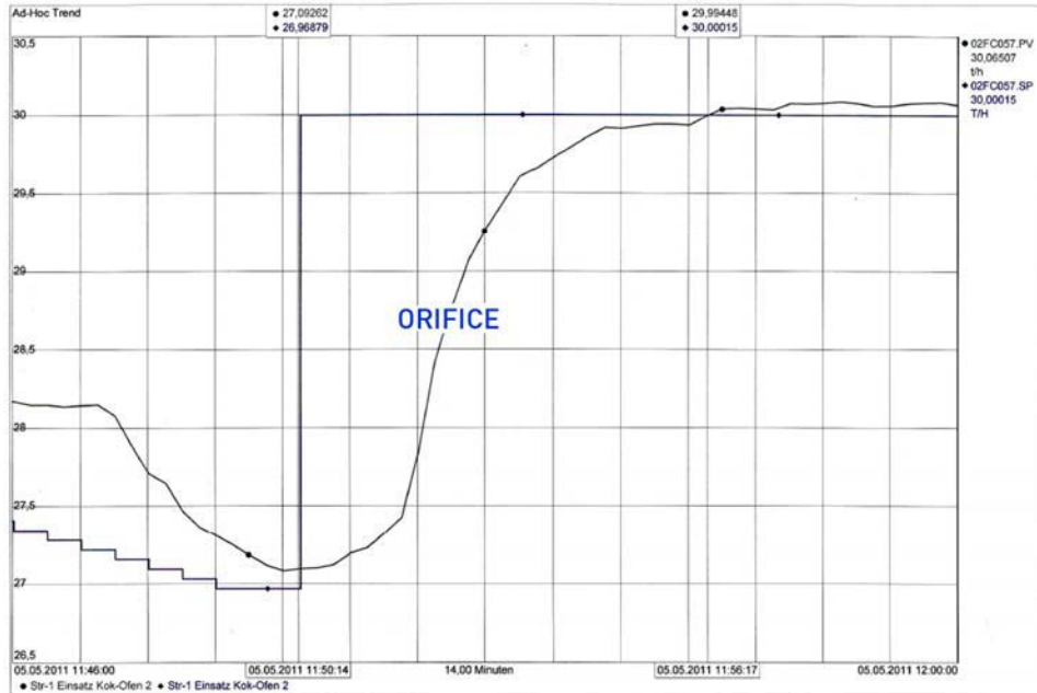
Fig. 22 : Comparison of the Control Behaviour of the \Delta p Flow Measurement
